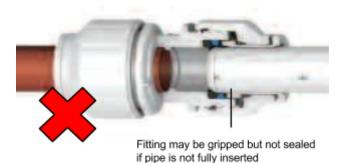
Don't forget to push the pipe fully into the fitting, past both the collet (gripper) and the 'O'.
