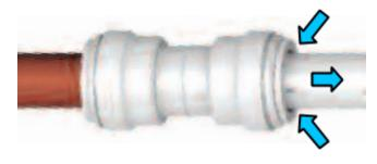
With the collet held in position the pipe can be removed.
