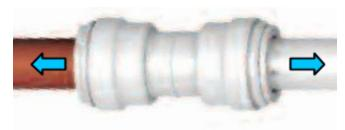
Pull to check the connection is secure. It is good practice to test the system prior to leaving the site or before use.
